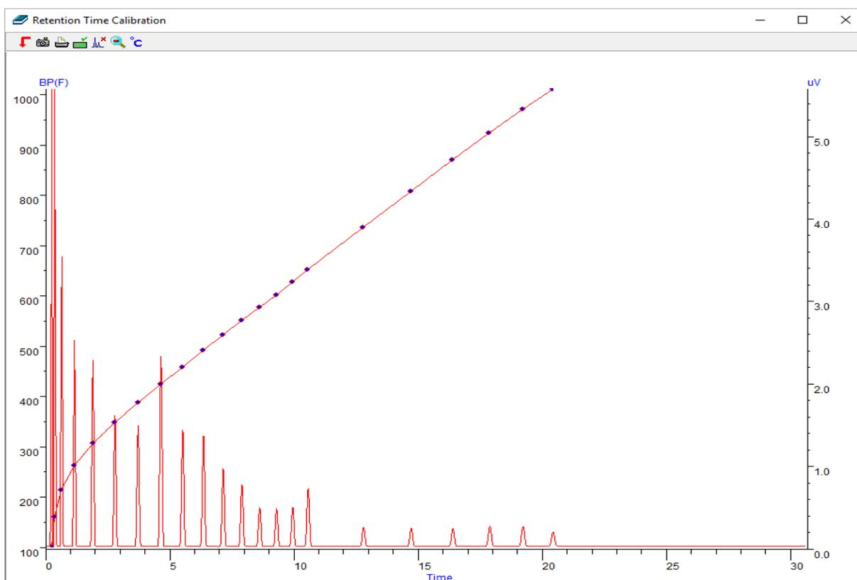
An example of a retention time calibration chromatogram with associated boiling point curve for ASTM D2887 (above) and the corresponding boiling point table with automatic skewness fit. (right)
